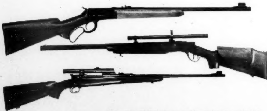
Other rifles popular with the small-game hunter are the Winchester model 65 (above), custom remodeled Sharps-Borchardt single-shot (center), and Winchester model 70 bolt action
